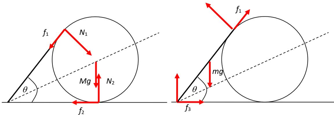
Taking torques about the center of the ring gives  $f_1 R = f_2 R$  and so we learn that  $f_1 = f_2 = f$ .
